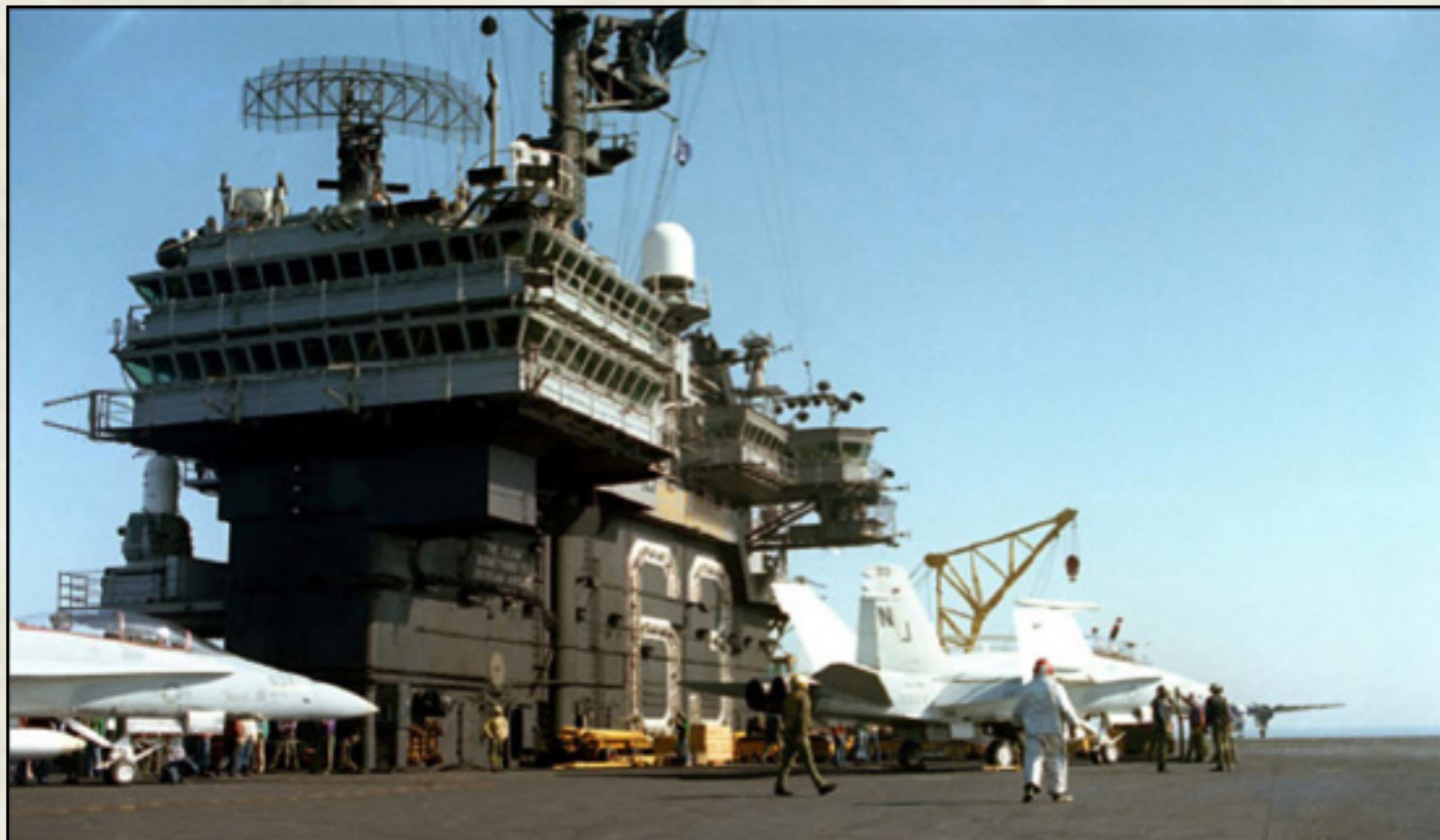
KEEPING TABS: The 'Island' on a Nimitz-class carrier. It is from this vantage point that the Air Boss and the Mini-boss keep a close eye on aircraft launching or landing on the deck.
