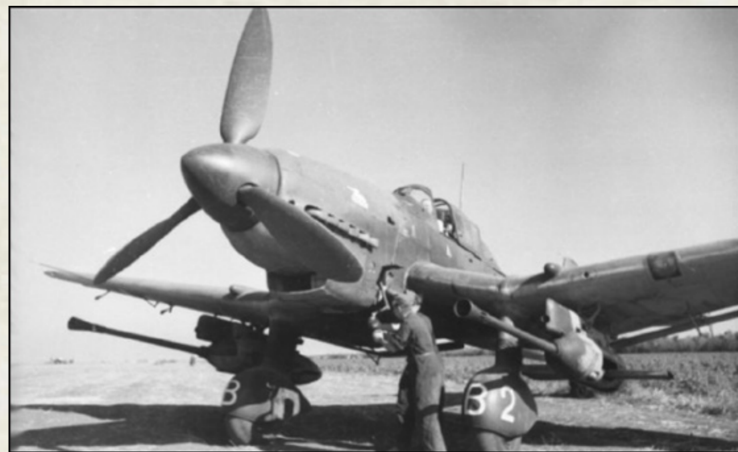
TANK KILLER: Hans-Ulrich Rudel's Junkers Ju 87G, with twin BK 3,7 gun pods attached to the underside of the wings, in Russia 1943.
