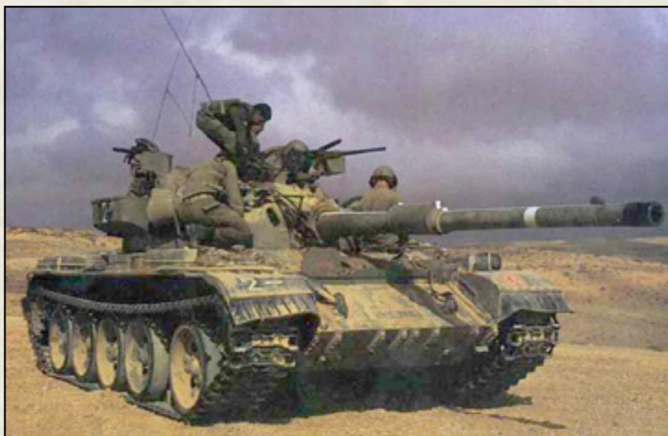
WOLF IN SHEEP'S CLOTHING: The Israeli Tiran-5 series of tanks were actually captured T-55 tanks. Most were captured from the Egyptian Army.
