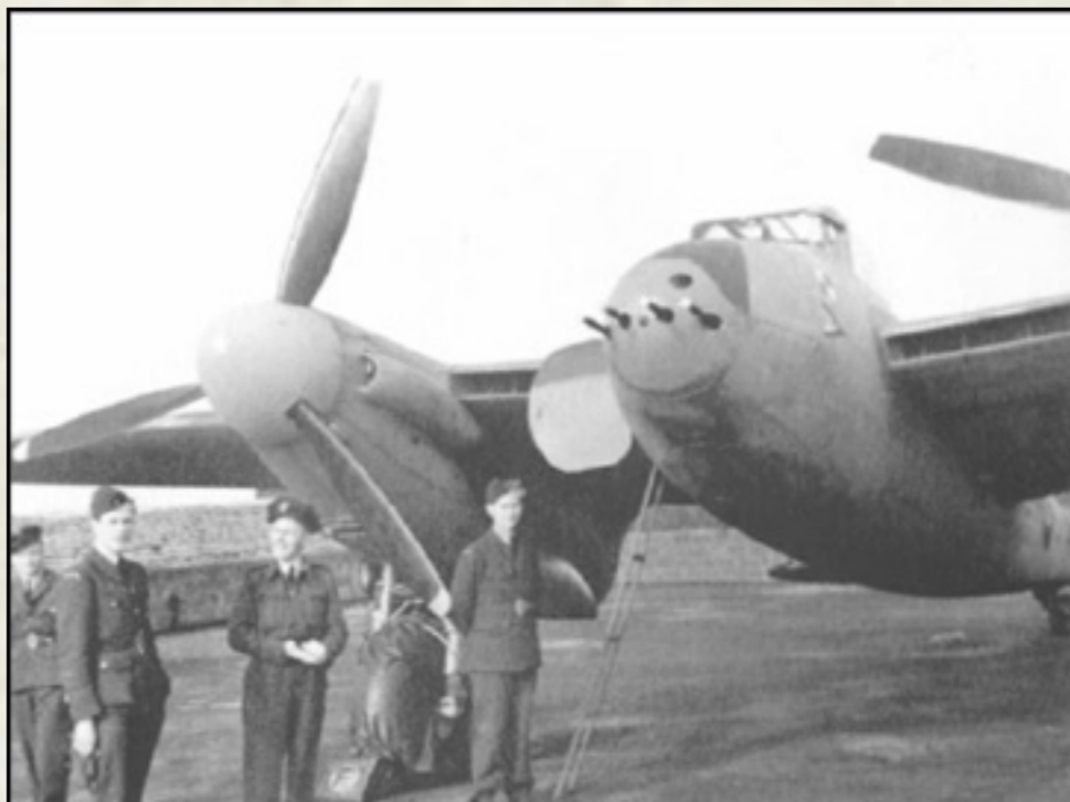
WOODEN WONDER: Pilots and crew pose in front of a Mosquito. Note the four .303 machine guns in the nose.
