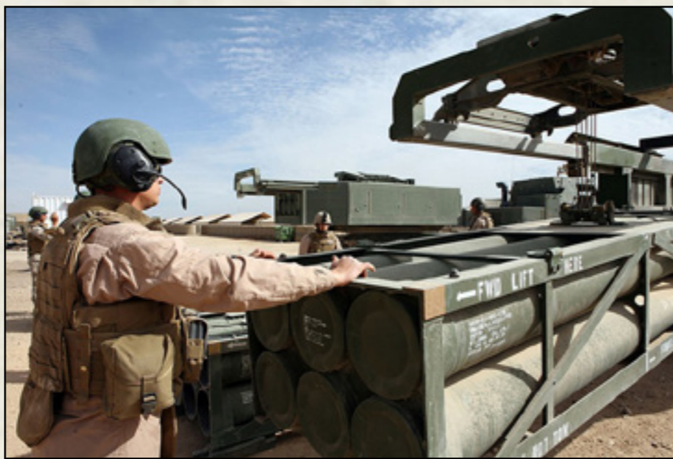
LOADED: A troop reloads a HIMARS with a pod of six rockets.
