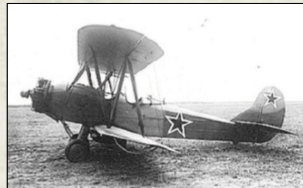
FLYING COFFIN: The Night Witches flew the Polikarpov Po-2, which was nicknamed the 'Flying Coffin'. Constructed from plywood and canvas it would often catch fire if hit by tracers.
